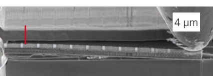
In-situ SEM nanomechanics cantilever experiment on a nanostructured microelectronics specimen.
